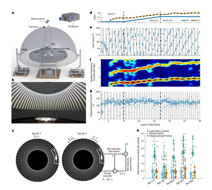
Stripe presentation and gain computation. a, Virtual reality Dome apparatus b, Stripes projected within the dome. c, Stripe gain, S, related the velocity of the rat
