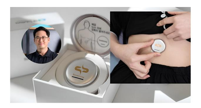
The image above shows Soomirang attached to the abdomen, a device designed to collect biometric data and analyze sleep patterns. l Credit: Professor Franklin Bien, Department of Electrical Engineering, UNIST
