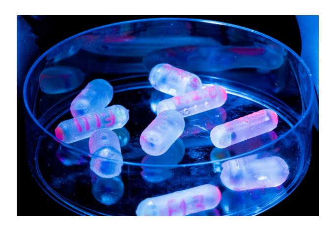
The pill devices have a soft elastic exterior with sidewall inlets, which are triggered to open by pH levels in the small intestine environment. Elastic microvalves close the inlets once the intestinal microbiome content has been collected. Credit: Sameer Sonkusale, Tufts University Nano Lab
