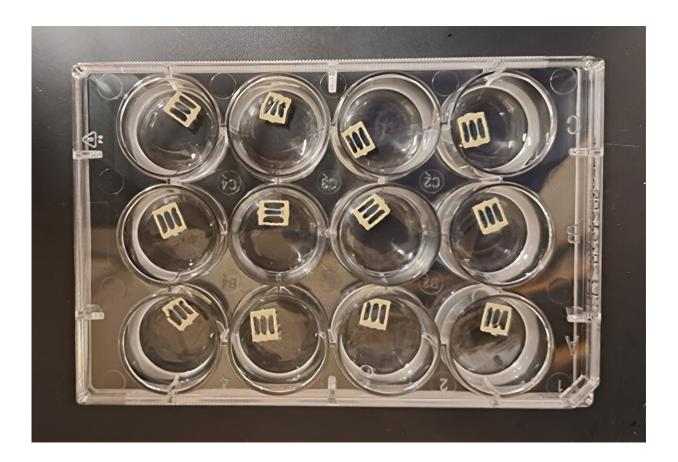
An array of Petri dishes each housing a platform for growing muscle fibers from stem cells. The Bursac Lab was the first to grow contracting, functional human skeletal muscle in a Petri dish and has been improving its processes ever since to enable studies of muscle strength, metabolism and repair. Credit: Alastair Khodabukus, Duke University
