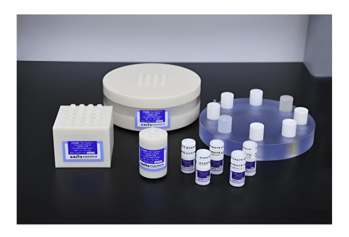
Emulsified reference material and phantom developed by KRISS for medical imaging devices. Credit: Korea Research Institute of Standards and Science (KRISS)
