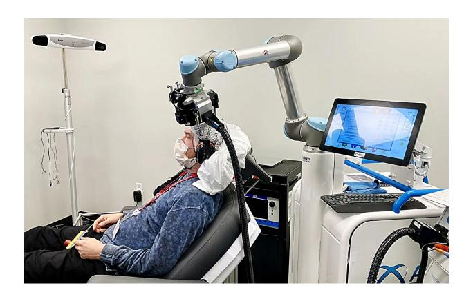
Brain electrical responses can be studied by measuring EEG simultaneously with brain stimulation. In the picture, a robotic arm holds the TMS coil. Credit: Juha Gogulski
