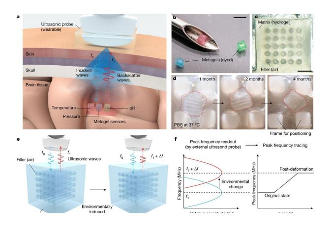
Design of injectable and biodegradable metagel ultrasonic sensor. a, Metagels as wireless intracranial physiology sensors using ultrasound reflection. b, Metagel samples and puncture needle for delivery. c, Metagel structure. d, Metagel degrading following 1 month in PBS solution at 37 °C; dashed line delineates the shape of the metagel. e, Working principle of metagels based on environment-induced microdeformation. f, Peak frequency shifts of metagel due to
