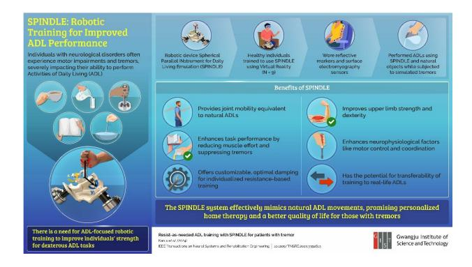
SPINDLE (Spherical Parallel INstrument for Daily Living Emulation) aims to help individuals with neurological disorders improve their upper limb strength, dexterity, and motor coordination by facilitating ADL training by mimicking natural movements and offering adjustable resistance levels. Credit: Jiyeon Kang from Gwangju Institute of Science and Technology
