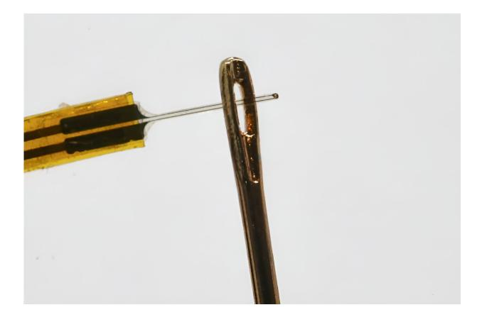
The new approach uses ultrasound delivered by a fiber about the thickness of a human hair. Credit: Massachusetts Institute of Technology
