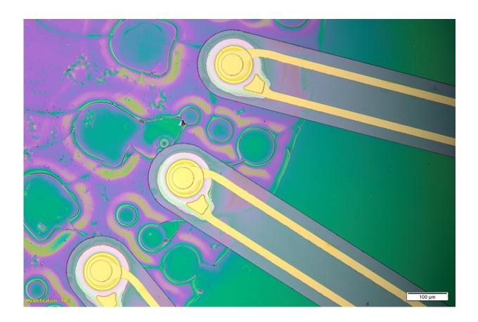
The ImPULS device contains ultrasound transducers and electrodes (gold) encapsulated within a polymer. Credit: Massachusetts Institute of Technology
