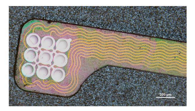
In the new system, transducers (silver) are powered by wires (gold) that deliver electrical stimulation. Credit: Massachusetts Institute of Technology
