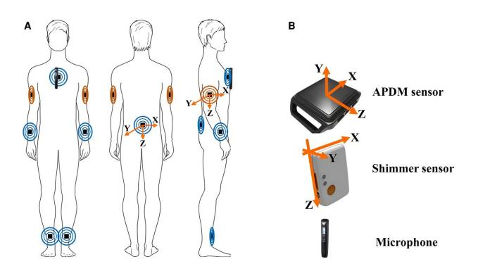
Sensor placement and orientation. (A) Shows the placement of APDM (in blue) and Shimmer (in orange) sensors, along with a microphone, on the human body. (B) Provides a detailed view of the sensors' orientation, indicating the axes' alignment for accurate data capture. Credit: *Frontiers in Digital Health* (2024). DOI: 10.3389/fdgth.2024.1366176
