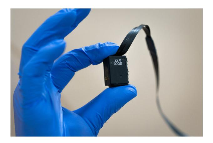
A researcher holds an Optically Pumped Magnetometer. Researchers have used these non-invasive devices to record, for the first time, activity in human cervical nerves. Credit: Qualcomm Institute/UC San Diego
