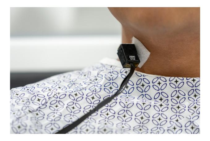
A researcher holds an Optically Pumped Magnetometer (OPM) to a person's neck. The OPMs can non-invasively measure neural activity in major nerves of the human neck, allowing researchers to track the body's inflammatory response. Credit: Qualcomm Institute/UC San Diego
