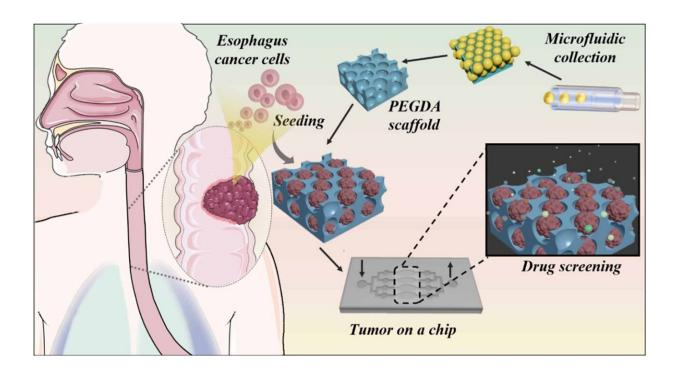
Schematic of microfluidic chip-based approach for quality assessment and screening of esophageal cancer drugs. A three-dimensional scaffold with inverse opal structure was fabricated using a single-emulsion microfluidic device. The esophageal cancer cells were loaded into the microfluidic chip to construct an esophageal cancer drug screening platform. Credit: *Materials Futures* (2024). DOI: 10.1088/2752-5724/ad5f47
