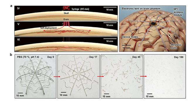
The process of shape recovery and biodegradation of the electronic tent. (a) Shape recovery process of the electronic tent in a skull and brain mimic model. (b) Biodegradation process of the electronic tent in phosphate buffered solution (PBS; 70°C, pH 7.4). Credit: Adapted from *Nature Electronics* (2024). DOI: 10.1038/s41928-024-01216-x
