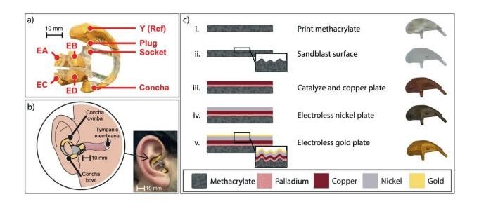
Earpiece assembly, fit, and manufacturing process. Credit: *Nature Communications* (2024). DOI: 10.1038/s41467-024-48682-7
