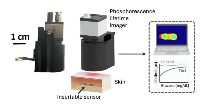
An insertable glucose sensor using a compact and cost-effective phosphorescence lifetime imager and machine learning. Credit: UCLA Engineering Institute for Technology Advancement
