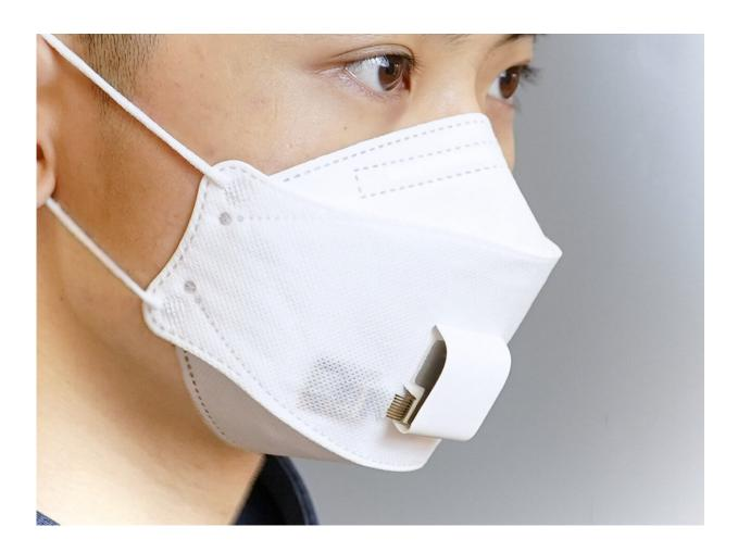
The EBCare mask can analyze the chemicals in one's breath in real-time. Credit: Caltech/Wei Gao and Wenzheng Heng
