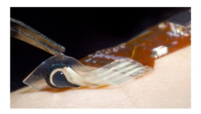
The sensor comprises an ionic electronic bilayer hydrogel that can detect solid state biomarkers from the skin. The sensor is connected to a flexible printed circuit board which transmits data wirelessly to a user interface. Credit: NUS iHealthtech
