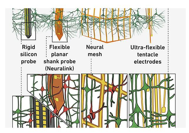
The tentacle electrodes (right) shown alongside three current technologies using thicker electrodes or an electrode mesh. Credit: *Nature Communications* (2024). DOI: 10.1038/s41467-024-49226-9
