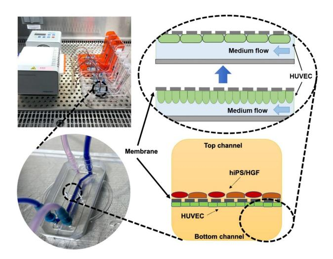
Perfusion system for the heart-on-a-chip. Endothelial cells are seeded in the bottom channel of the microfluidic chip, while induced pluripotent stem cells and fibroblasts are seeded in the top channel. The culture medium is delivered by
