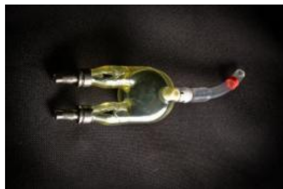
The Berlin Heart, a pediatric heart pump, seen on the side where the blood chamber is located. Credit: Jacobs School of Engineering at UC San Diego
