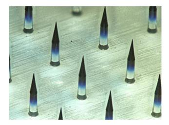
A micro-needle array injected with pigments instead of drugs. Drugs can be injected into the projections (L1000µm x D170µm).
