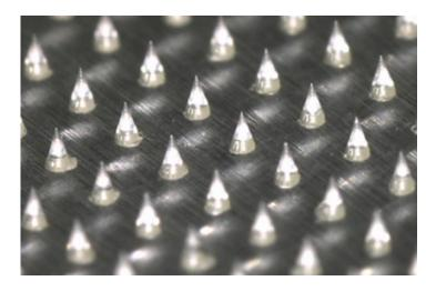
A sample of Fujifilm's micro-needle array (L500µm x D200µm).
