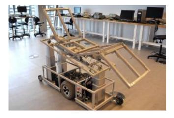
The Flexbed incorporates the movements of seven existing hospital bed types.
