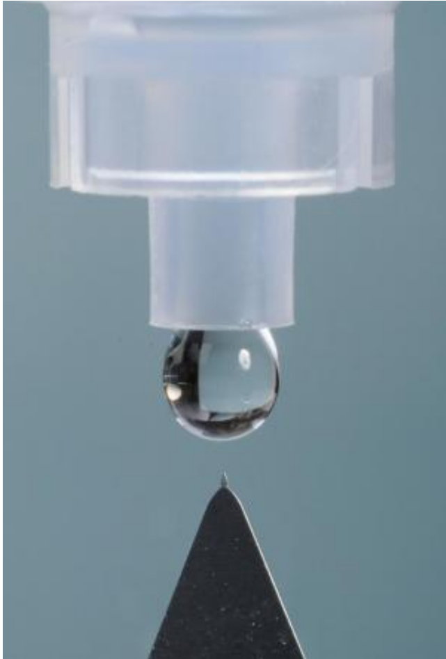
A solid microneedle coated with medication for delivery into the cornea is shown next to a liquid drop from a conventional eye dropper. Credit: Georgia Tech Photo: Gary Meek
