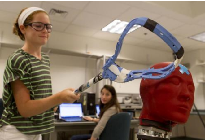
A girls' lacrosse player wallops a headform in the lab as part of a study of the acceleration imparted to the head by such stick blows. Credit: Michael Cohea/Brown University
