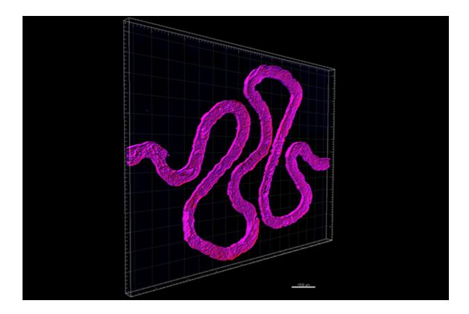
Using fugitive ink, a convoluted hollow channel is fabricated to mimic the winding shape of natural proximal tubules found inside a human kidney's nephrons. Credit: Lewis Lab/Wyss Institute at Harvard University.
