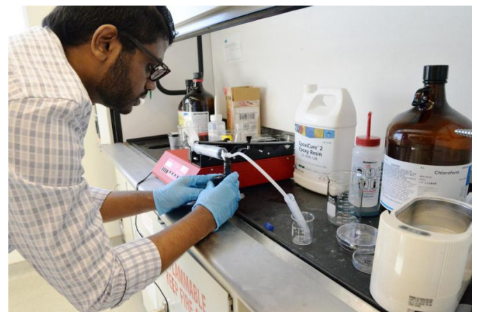
Suraj Kandalam, a biomedical engineering graduate student, works with a pump to infuse e-liquid vapor with saline to use during experimentation. The pump, which he created by modifying an apparatus that mimics smoking tobacco cigarettes, is meant to realistically simulate vaping. An atomizer heats up the e-liquid, turning it into vapor, which is then sucked through a syringe before it is infused with the saline. Credit: Leah Small, University Public Affairs
