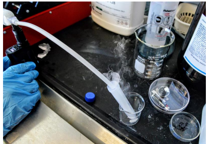
E-cigarette vapor rises from a beaker while researcher Suraj Kandam demonstrates the use of a pump meant to simulate e-cigarette smoking and to create solutions used in testing. Credit: Leah Small, University Public Affairs
