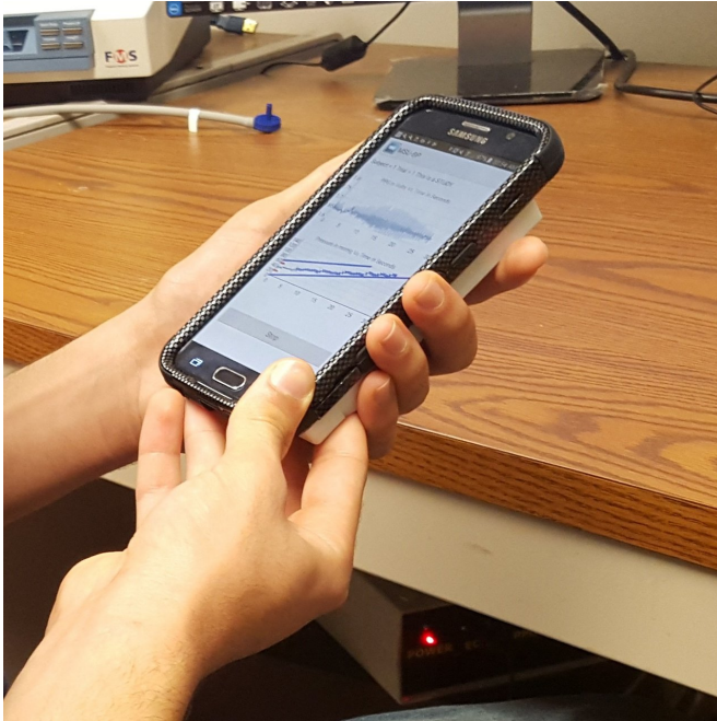
Smartphone based device for real-time monitoring of BP. Credit: Anand Chandrasekhar
