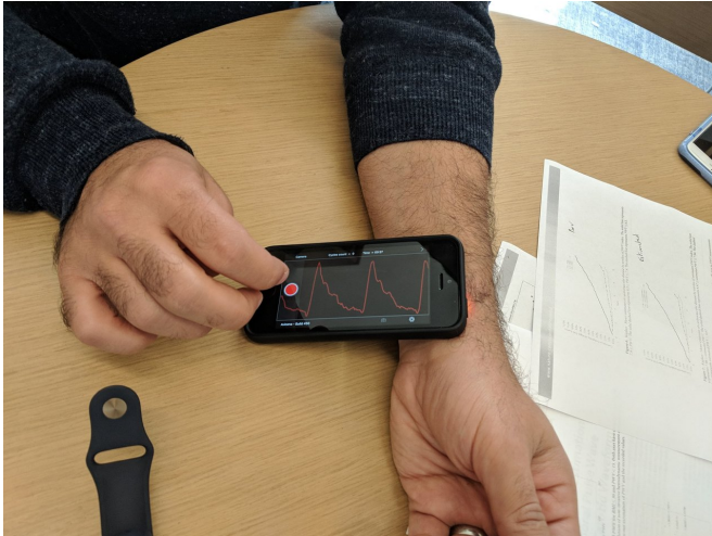
Assistant Professor Niema Pahlevan demonstrating their iPhone app's ability to capture a pulse wave using just the phone's camera. Credit: Ashleen Knutsen
