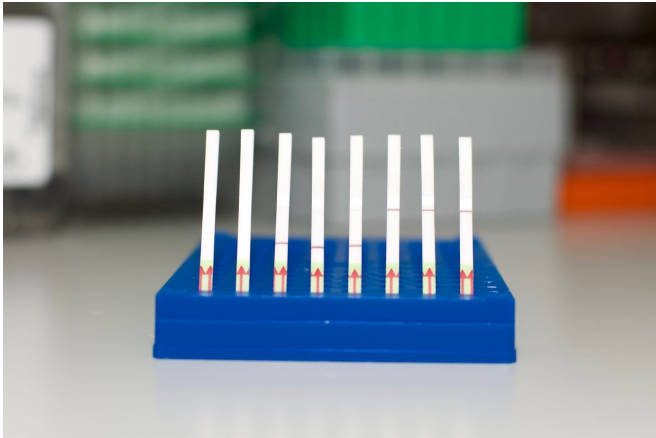
A collection of SHERLOCK paper test strips. (Left) Unused paper strips. (Middle) Paper tests displaying a negative SHERLOCK readout. (Right) Paper tests displaying a positive SHERLOCK readout. Credit: Broad Institute of MIT and Harvard
