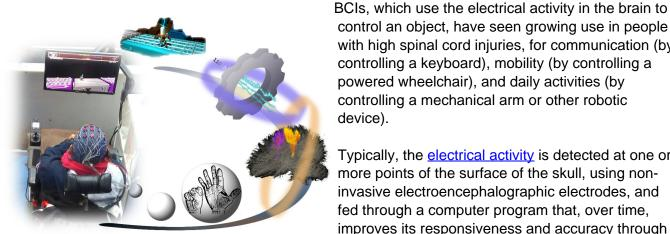
powered wheelchair), and daily activities (by controlling a mechanical arm or other robotic device). Typically, the <u>electrical activity</u> is detected at one or more points of the surface of the skull, using noninvasive electroencephalographic electrodes, and
