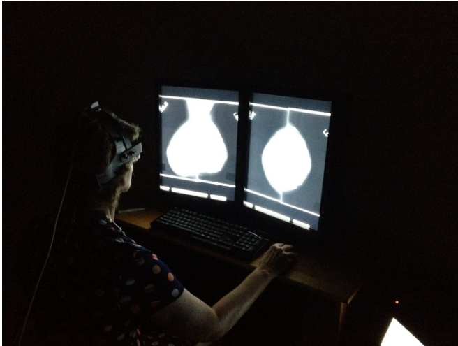
A radiologist outfitted with the team's head-mounted eye-tracking device examines a mammogram. Credit: Hong-Jun Yoon/Oak Ridge National Laboratory, U.S. Dept. of Energy
