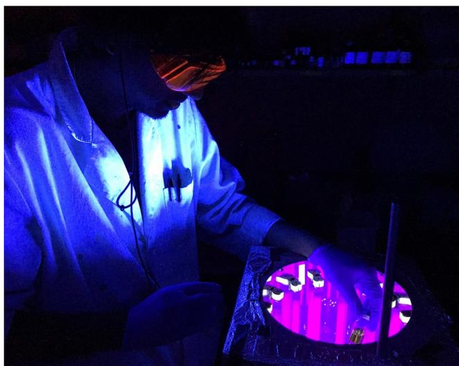
Charitha Guruge, a Ph.D. student at Florida Institute of Technology, places a sample of an inactive, or "caged," version of the neurotransmitter glutamate in a photo reactor. The UV lamps in the reactor activate the neurotransmitter, which is a key tool for neuroscientists to use in mapping the enormously complex brain circuitry. Credit: Florida Institute of Technology
