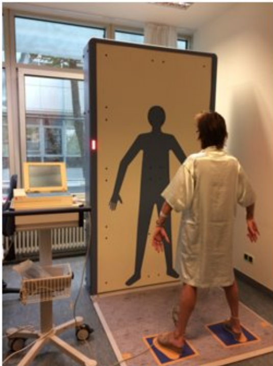
Millimetre wave body scanner at the German Heart Centre Munich Credit: German Heart Centre Munich with the patient's written consent.
