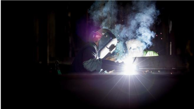
The fume generated during arc welding is detrimental to human health because of dangerous nanoparticles contained in it. Credit: Photo captured by Pete Wright, @petewright
