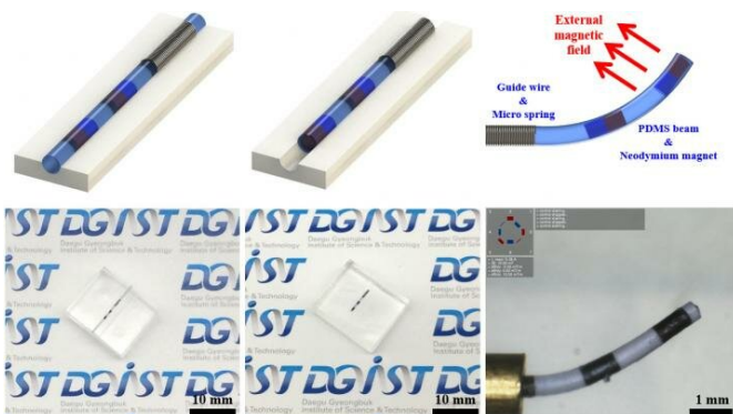
Manufacturing process and concept map of attachable guidewire microrobot, actually manufactured microrobot Credit: ©DGIST
