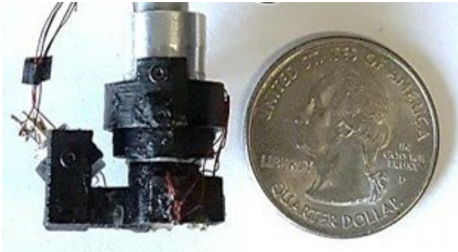
The mini microscope measures 5 cubic centimeters - smaller than a US quarter. Credit: Arvind Pathak
