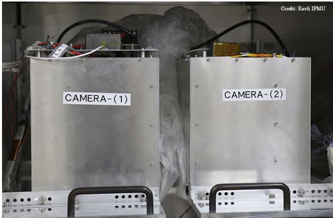
Compton camera being tested at Kavli IPMU. Credit: Kavli IPMU
