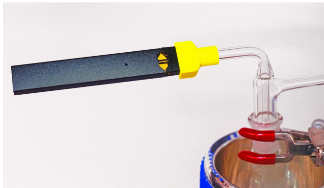
A Yale-designed machine captures Juul aerosol to determine its chemical makeup. Credit: Hanno Erythropel
