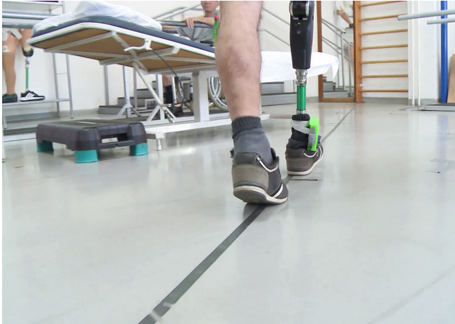
Volunteer finely places the prosthesis with feedback on the straight line. Credit: Francesco M. Petrini
