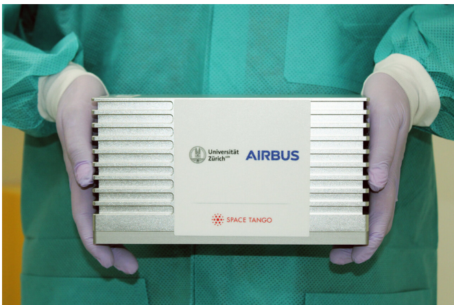
Housing of the mobile CubeLab containing 250 test tubes for the production of human tissues in weightlessness. Credit: Space Tango
