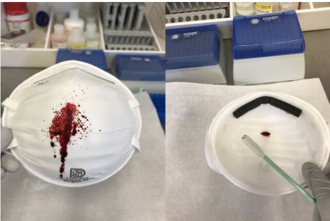
The laboratory is using synthetic blood to test surgical-grade N95 and similar respirator masks' resistance to blood spatter. Here, a mask has failed the test, as the liquid has soaked through to the other side. Credit: Massachusetts Institute of Technology
