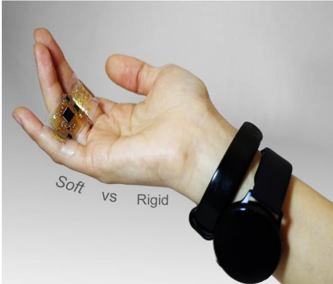
How the wearable sleep monitoring device compares to wearable body movement monitors. Credit: W. Hong Yeo
