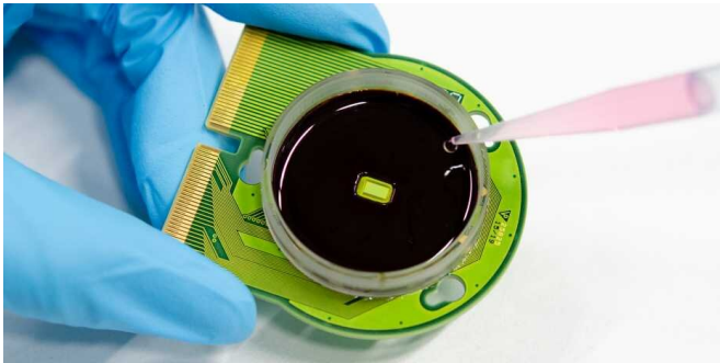
Measuring chip at the base of a cell-culture dish. Credit: ETH Zurich / Xinyue Yuan
