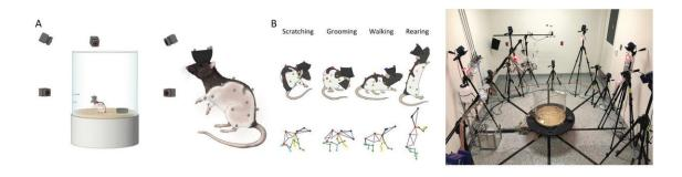
We equip a rat with 20 retrore\_ective markers that are chronically attached using body piercings. These markers are attached using a 12 camera array, allowing us to reconstruct the animals' full pose across a diverse range of behaviors. Credit: BP Ölveczky & JD Marshall
