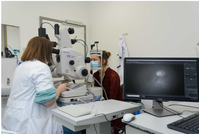
Setup of combined hyperspectral and fundus camera at Stalmans' lab. Credit: IMEC
