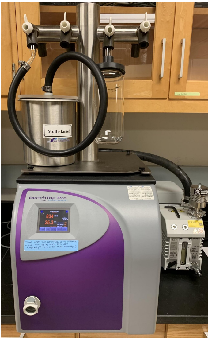
A lyophilizer, the instrument used to freeze-dry diagnostics. Credit: Northwestern University
