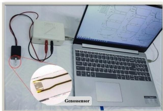
Impedance analyzer connected to DNA biosensor that can be used to detect genetic sequence from SARS-CoV-2. Credit: Lorenzo A. Buscaglia/IFSC-USP
